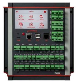
The local interface between the operator and the Compact and Compact Plus dataloggers is simple and intuitive, comprising a 4.3" **DTS** (Display Touch Screen), **capacitive** and **multi-touch** terminal. The display allows **full control over the tasks of the datalogger**: internal operation status, data acquisition, display of charts and tables, connection with external modules. **Furthermore**, it allows running a wizard to configure the station, maintaining its integrity.
