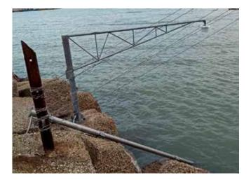
**pyranometer and a water quality probe**, such as the one installed at the Po River in Pontelagoscuro for ADBPO and ARPAE (please, find here the related links).
