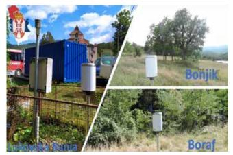
Thanks to the **low consumption**, **standard batteries** guarantee **uninterrupted operation** for very long periods of time and, at the same time, highly simplify installation operations. PG4i do not require solar panels or mains electric power supply.
