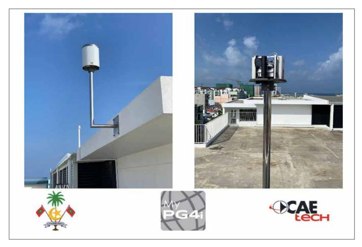
PG4i are autonomous rain gauges with a collection surface of 400 cm<sup>2</sup> which, thanks to an integrated 3G modem, are able to measure, locally record and autonomously send data relating not only to **accumulated rainfall**, but also to its **intensity per minute** to an FTP server, all without any connection to an external datalogger.
