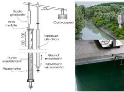
The radar hydrometer was compared to the primary system of the Hydraulic Engineering Laboratory of the University of Bologna as far as the measurement of liquid levels. The test environment consists of a calibration tank
